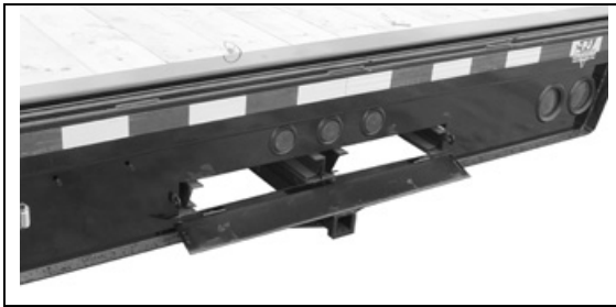
Rear Storage Position Ramps – Figure 6-9
